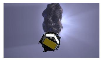
infrared spectrometer, which comprise the High Resolution Instrument, are carried on the flyby spacecraft, along with a Medium Resolution Instrument. A duplicate of the Medium Resolution Instrument on the impactor will record the vehicle's final moments before it is run over by Tempel 1.
