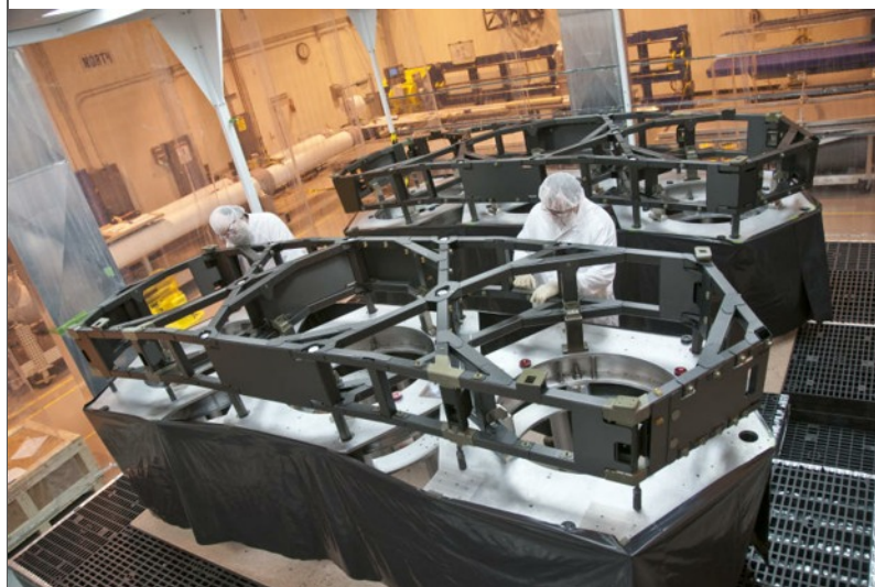
Technicians complete the primary mirror backplane support structure wing assemblies for NASA's James Webb Space Telescope at ATK's Space Components facility in Magna, Utah. ATK recently completed the fabrication of the primary mirror backplane support structure wing assemblies for prime contractor Northrop Grumman on the Webb telescope. (Credit: Northrop Grumman/ATK)
