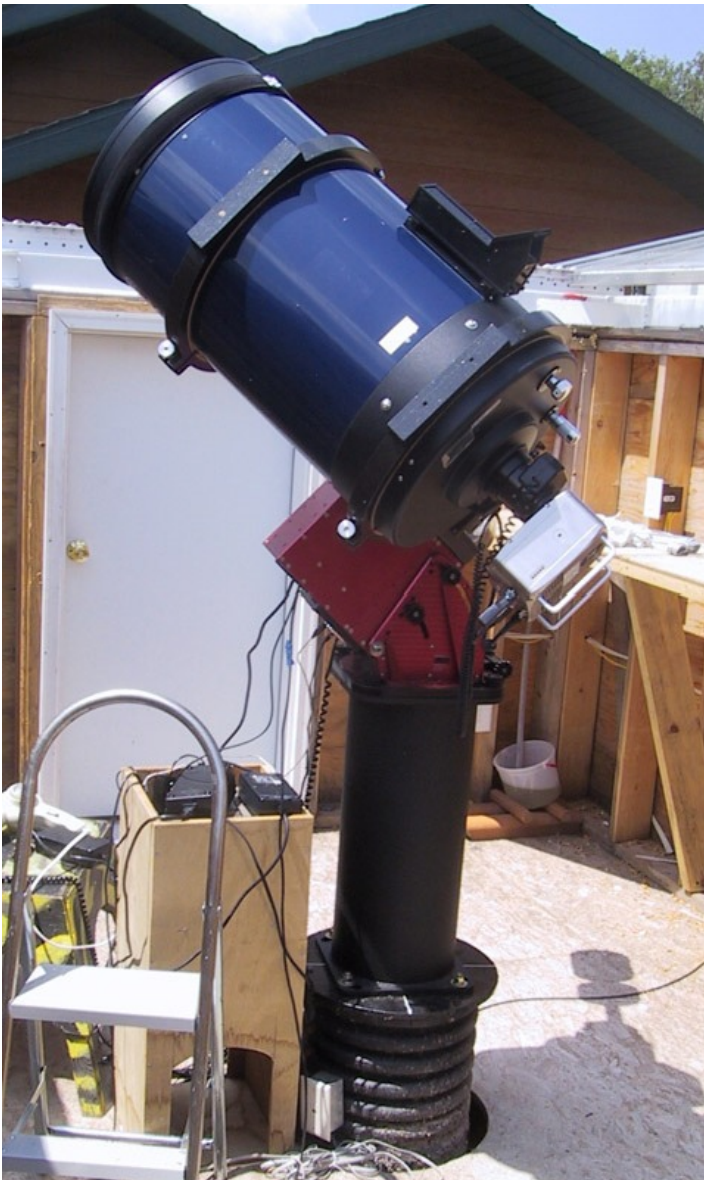
14" system as first configured with the inadequate Meade focuser.
