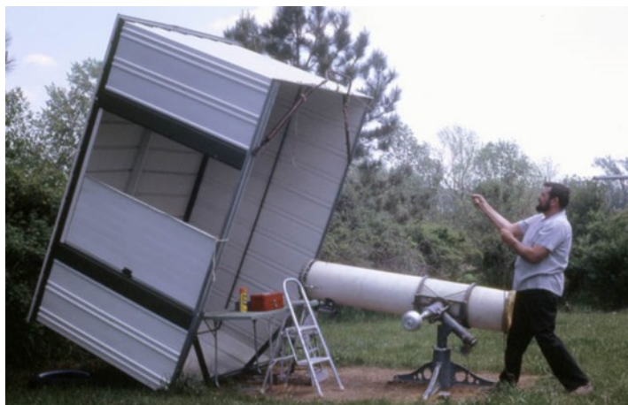
Earl opening the club's tip off observatory housing a 12.5" f/7 reflector in his back yard about 1967 judging by his beard. He grew one for the Nebraska Centennial that year.
