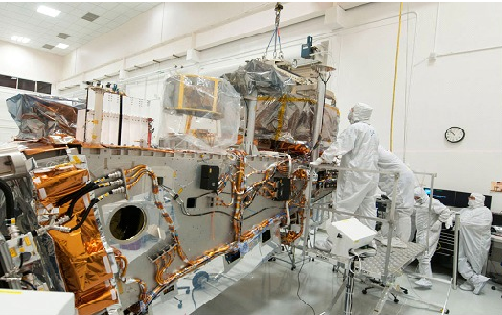
Caption: Ball and Raytheon technicians integrate the VIIRS Optical and Electrical Modules onto the JPSS-1 spacecraft in 2015. The spacecraft will be ready for launch later this year. Image Credit: Ball Aerospace & Technologies Corp.
