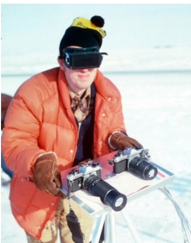
Donn Baker with of #14 dark welders goggles and a home-made tracking platform on which he had mounted two cameras.
