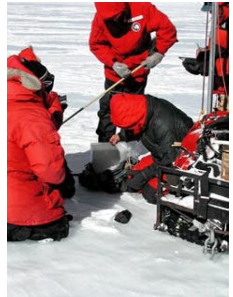
Recovery of a meteorite in Antarctica by members of the Antarctic Search for Meteorites (ANSMET) expedition. A meteorite is picked up with sterile tongs and put into a clean Teflon bag. NASA
