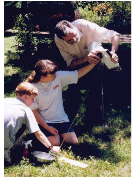
Above Left: Liz Klimek holds the mirror blank while John Dowd wets the surface with water from a squirt bottle. Above Right: Michael and Margaret Fairchild measure the distance from the wet mirror to the image of the sun on a piece of paper held by Martin Gaskell.
