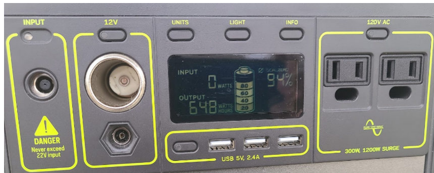
Power connectors and status display of the Goal Yeti 400
