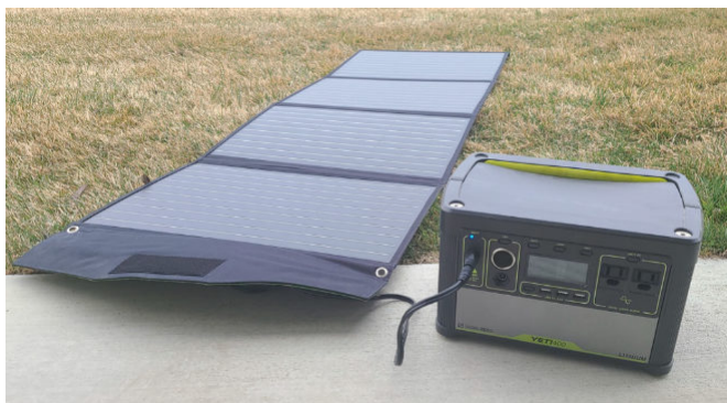
The TwelSeavan Portable 120W Solar Panel Charger. I found this foldable panel on Amazon. It has three USB ports and a 12V barrel connector with adapter cable that matches the 12V input on the Yeti.
