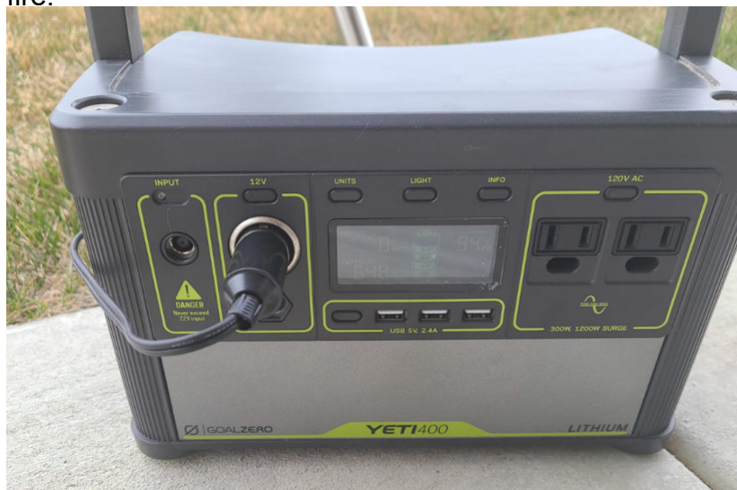
The Goal Zero Yeti 400 Lithium Ion Power Station Rated at 428Wh, pure sine wave, 300W continuous, 1200W surge max
