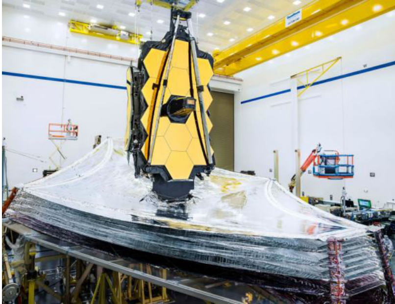
During a test, engineers and technicians fully deployed all five layers of the James Webb Space Telescopes sunshield. Image Credit: NASA/Chris Gunn
