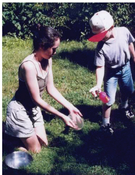
Right: Michael and Margaret Fairchild measure the distance from the wet mirror to the image of the sun on a piece of paper held by Martin Gaskell.
