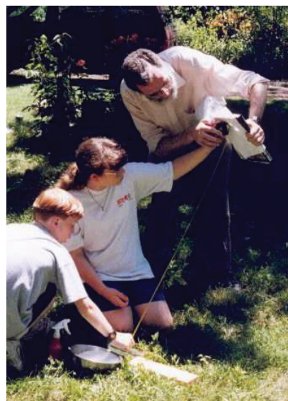
Right: Michael and Margaret Fairchild measure the distance from the wet mirror to the image of the sun on a piece of paper held by Martin Gaskell.
